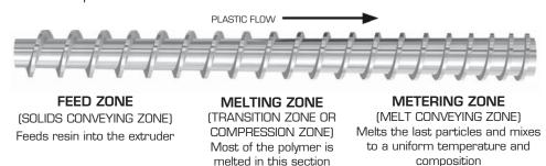
Determining the ultimate length of a screw for production involves using the proper length to diameter (L:D) ratio. For example, a typical 6" diameter screw at a 24:1 ratio will be 144" (12') long, and at a 32:1 ratio it is 192" (16') long. An L:D ratio of 25:1 is common, but some machines go up to 40:1 for more mixing and more output at the same screw diameter.
